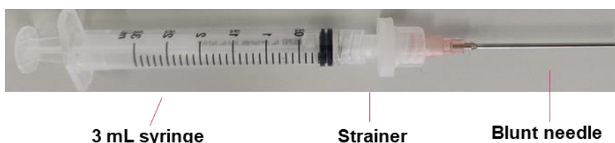
Figure 4-1 Load cells into 3 mL syringe with strainer and blunt needle.
