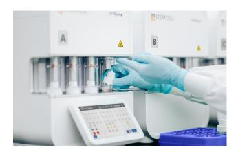
i) Initially, the Run Control screen will display a dimmed sample tube icon ② for the empty slot (to indicate that no sample tube is present). Insert a STEMprep™ Sample Tube in the slot; the icon will change to indicate a sample tube is present ③.
