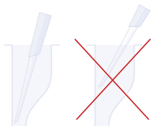
Figure 1. Proper Pipetting Technique for CellPore™ Delivery Cartridge 300
