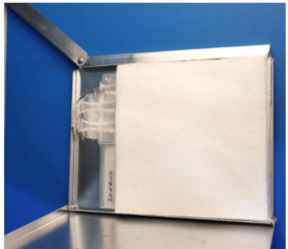
6. For 50ml cryobags that have a flap extension feature, the flap should be on the topmost side during freezing as shown in **Figure 3**.
