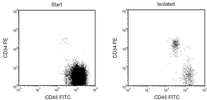
Starting with whole blood, the CD34+ cell content of the enriched fraction typically ranges from 26 - 41% (95% CI; reported as a percentage of viable CD45+ cells). In the above example, the purities of the start and final isolated fractions are 0.09% and 40%, respectively. RBCs were lysed prior to flow cytometry.
