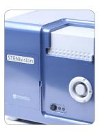
Automated colony scoring may help to standardize CFC assays within and between laboratories providing uniform consistent colony scoring criteria. STEMvision™. developed STEMCELL Technologies, is the first instrument and computer platform for imaging and automated scoring of hematopoietic colonies in CFC assays using MethoCult™ media. STEMvision™
